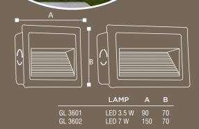
Lighting technology Luminaries with LED Lamp With LED Integral Power Supply unit
